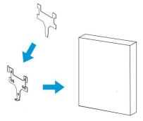
2. Put the device on the mounting bracket, then fix the bottom of the device to the bracket with the theft-deterring screw.
